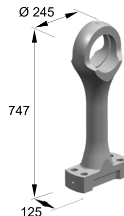
Connecting rod shaft (Weight : approx. 71.36 kg)
