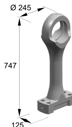
Connecting rod shaft (Weight : approx. 71.36 kg)
