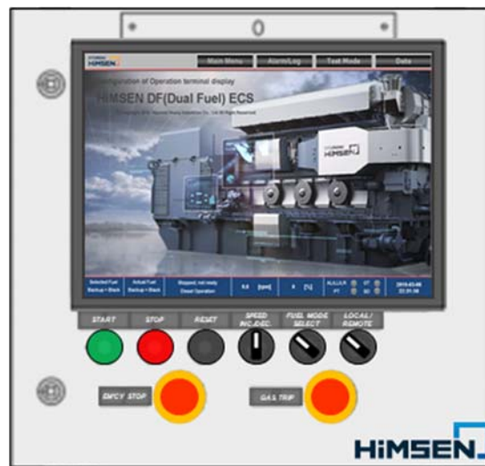
Figure 5.15 Local operating panel
