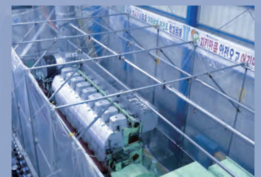
Water Spray Test for Kori #1 EDG
