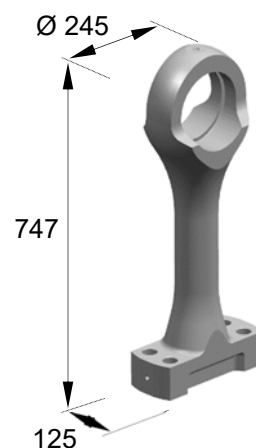
Connecting rod shaft (Weight : approx. 71.36 kg)
