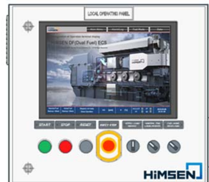
Figure 5.15 Local operating panel
